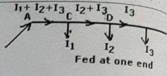
the number of load points e) Current in any section is equal to the sum of all load currents less sum of the load currents previous to the section, f) The voltage drop in any section is the product of current in that section and the resistance of that section for both go and return conductor.
