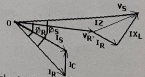
phase of the three phase line. The vector diagram also is shown.  $I_R$  is the load current per phase and receiving end lagging pf =  $\cos \phi_R$ . R and  $\mathcal{X}_L$  are the resistance and inductive reactance per
