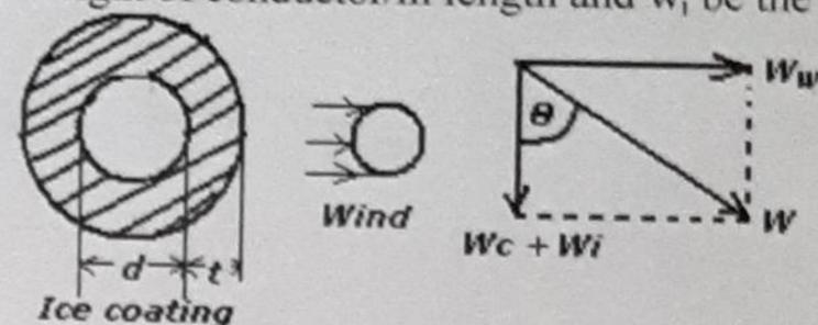
Is acting at an angle  $\theta = \cos^{-1} \frac{w_c + w_i}{w}$ . For ice coating and wind load the sag calculated is slant at an angle  $\theta$  to the vertical. Vertical sag = slant slag x cos  $\theta$ .
