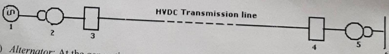
a) Alternator: At the generating station generating voltage of alternators is at 11kV.
