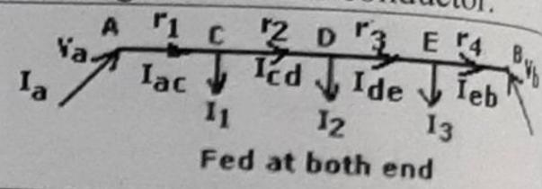
The point of minimum voltage is the point where current from both sides meet.
