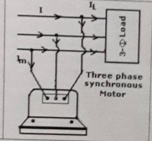
synchronous motor is not self starting an auxiliary starting device is required.
