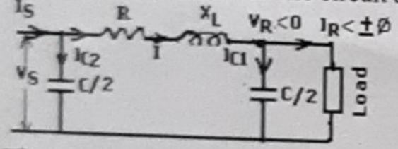
$\overrightarrow{l_R} = I_R(\cos \emptyset_R - j \sin \emptyset_R). \overrightarrow{I_{C1}} = j \frac{2\pi f C V_R}{2} =$  $j\pi fCV_R$ ;  $\vec{l} = \vec{l}_R + \vec{l}_{C1}$ ;  $\vec{V}_S = V_R + \vec{l}(R + jX_L)$ .
