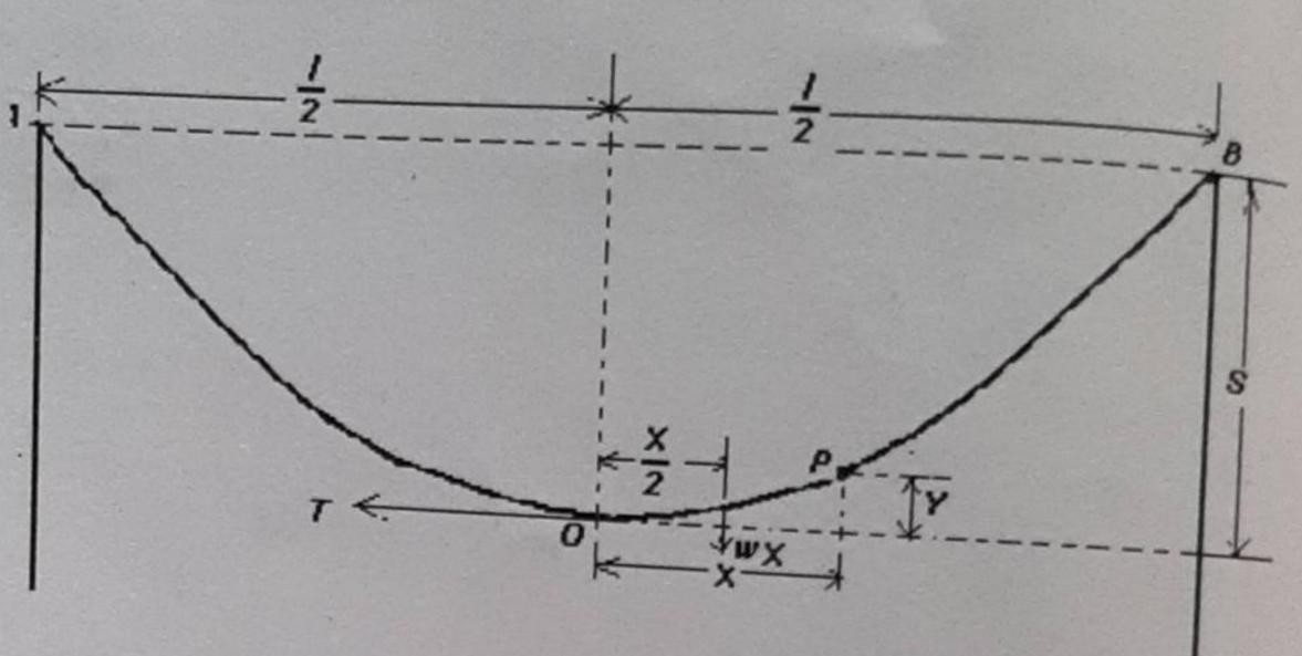
Taking O as the origin consider a point P on the conductor whose coordinates are x and y. The curvature of OP being very small we can take  $OP \cong x$ . The forces acting on OP are i) T at O and ii) wx at  $\frac{x}{2}$  from O. In order that P is is equilibrium the moments of these two forces about P must be equal. So  $Ty = wx \cdot \frac{x}{2} = \frac{wx^2}{2}$  or  $y = \frac{wx^2}{2T}$  When  $x = \frac{1}{2}$ , sag is maximum (S). So maximum sag
