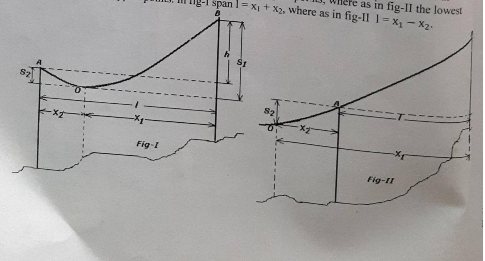
Referring to Fig-I,  $S_1 = \frac{wx_1^2}{2T}$  and  $S_2 = \frac{wx_2^2}{2T}$ .  $x_1 + x_2 = 1...(i)$  Now  $S_1 - S_2 = h = \frac{w}{2T}(x_1^2 - x_2^2)$  $(x_1^2) = \frac{w}{2v}(x_1 + x_2)(x_1 - x_2) = \frac{wl}{2T}(x_1 - x_2)$  or  $(x_1 - x_2) = \frac{2T(S_1 - S_2)}{wl} = \frac{2Th}{wl}$ ...(ii) Solving eq. (i) and (ii)  $x_1 = \frac{1}{2} + \frac{Th}{wl}$  and  $x_2 = \frac{1}{2} - \frac{Th}{wl}$ . Note that if value of  $x_2$  comes –ve then point O is
