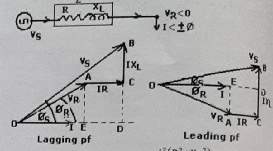
$$V_{S} = \sqrt{[V_{R}^{2} + I^{2}(R^{2} + X_{L}^{2}) + 2V_{R}(IR\cos\phi_{R} \pm IX_{L}\sin\phi_{R})]} = V_{R}[1 + \frac{I^{2}(R^{2} + X_{L}^{2})}{V_{R}^{2}} + \frac{I^{2}(R^{2} + X_{L}^{2})}{V_{R}^{2}}] + \frac{I^{2}(R^{2} + X_{L}^{2})}{V_{R}^{2}} + \frac{I^{2}(R^{2} + X_{L}^{2})}{V_{R}^{2}} + \frac{I^{2}(R^{2} + X_{L}^{2})}{V_{R}^{2}}] + \frac{I^{2}(R^{2} + X_{L}^{2})}{V_{R}^{2}} + \frac{I^{2}(R^{2} + X_{$$
