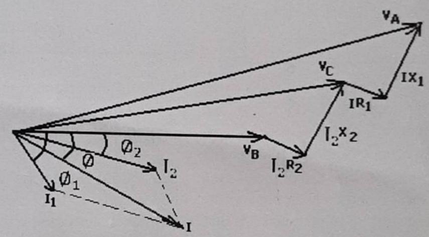
vector diagram is also shown.  $V_B$  is taken as reference.  $\vec{V_C} = V_B + \vec{I_2}(R_2 + jX_2) = V_B + I_2(\cos \phi_2 - j \sin \phi_2)(R_2 + jX_2)$ .  $\vec{I} = \vec{I_2} + \vec{I_1}$ ,  $\vec{I_1} = I_1(\cos \phi_1 - j \sin \phi_1)$ .  $\vec{V_A} = V_C + \vec{I_1}(R_1 + jX_1)$
