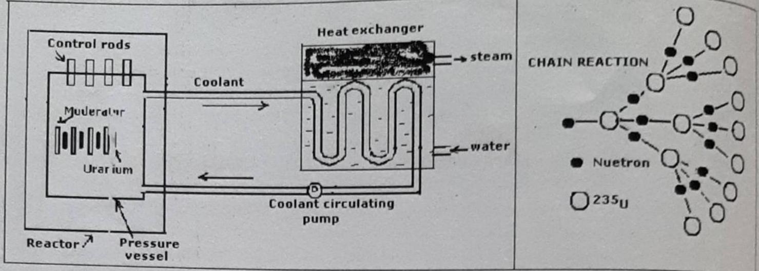
reactor the moderator slows down the neutrons before they hit the fuel rods and the cadmium control rods absorb the neutrons and controls the number of neutrons bu pushing the rods up and down as per requirement.
